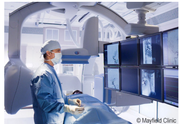
Figure 2. A fluoroscopic C-arm is an arc-shaped piece of equipment that generates x-rays from one side and photographs them on the other side.
